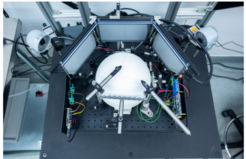
Mice are expert visual navigators— doing so more efficiently and reliably than the best human-made technology. To study how brain circuitry supports this expert behavior, researchers have mice walk on a spherical treadmill surrounded by screens displaying a virtual reality (VR) environment.
